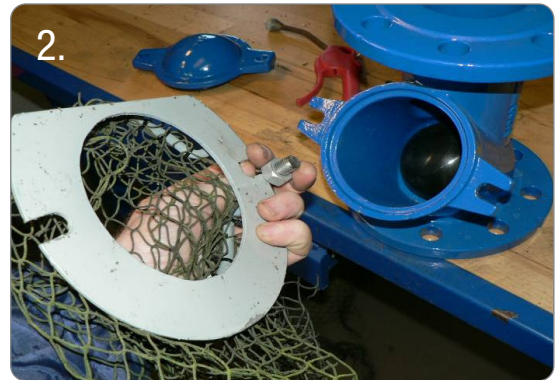
Mount the flange and net
