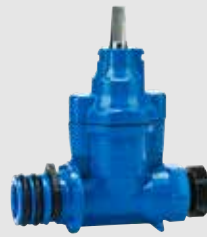
Series 103/50 - Service connection valve with one Supa Lock™ spigot end and one PRK coupling end, ductile iron.
